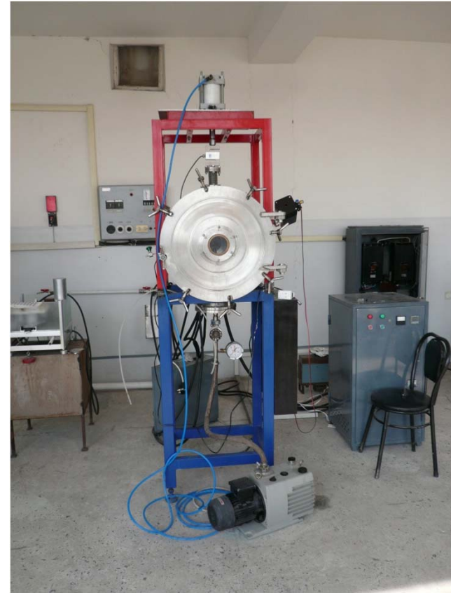
Diffusion welding machine (induction)
