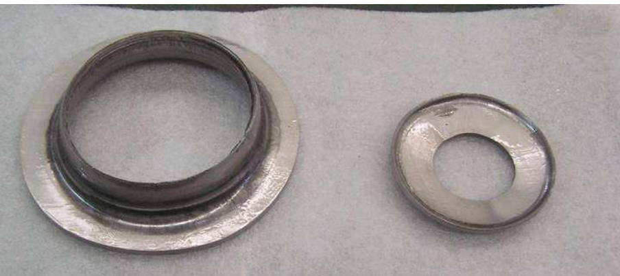
Broken part of beam-pipe transition
