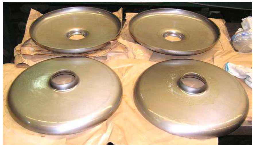
Half-cell after deep drawing.
