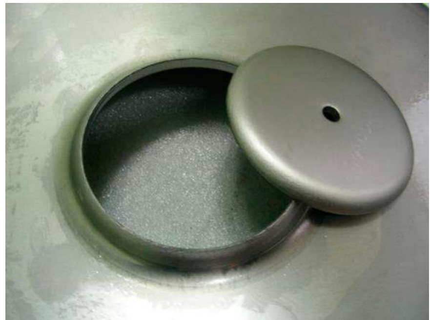
Broken part of half-cell during deep drawing
