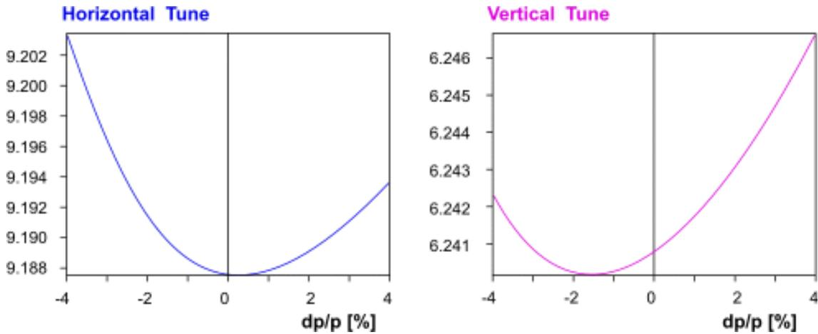
**Fig. 4.2.4 Momentum dependent tunes of the booster at extraction energy 3 GeV.**
