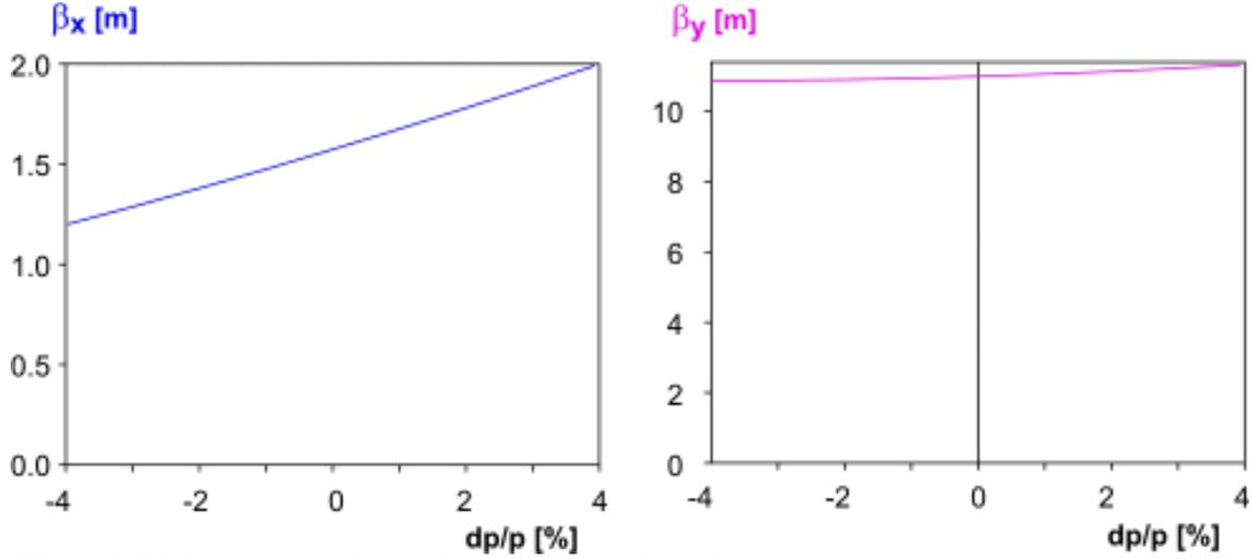
Fig. 4.2.5 Momentum dependence of beta functions at the extraction energy 3 GeV.
