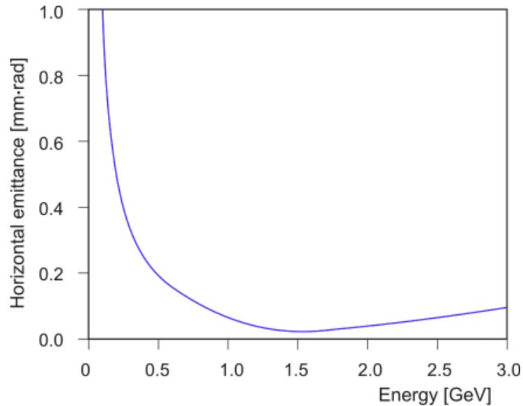
**Fig. 4.2.1 Evolution of the beam horizontal emittance during ramping. The minimum emittance of about 30 nm-rad is reached at an energy of 1.5 GeV.**
