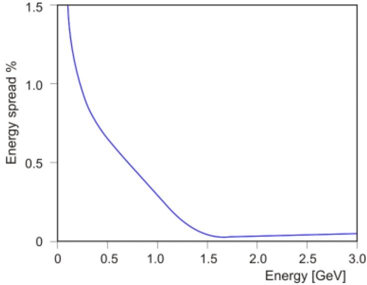
**Fig. 4.2.3 Beam rms energy spread variation during acceleration process.**
