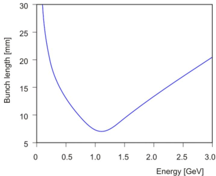
**Fig. 4.2.2 Bunch rms length variation during the energy ramp.**
