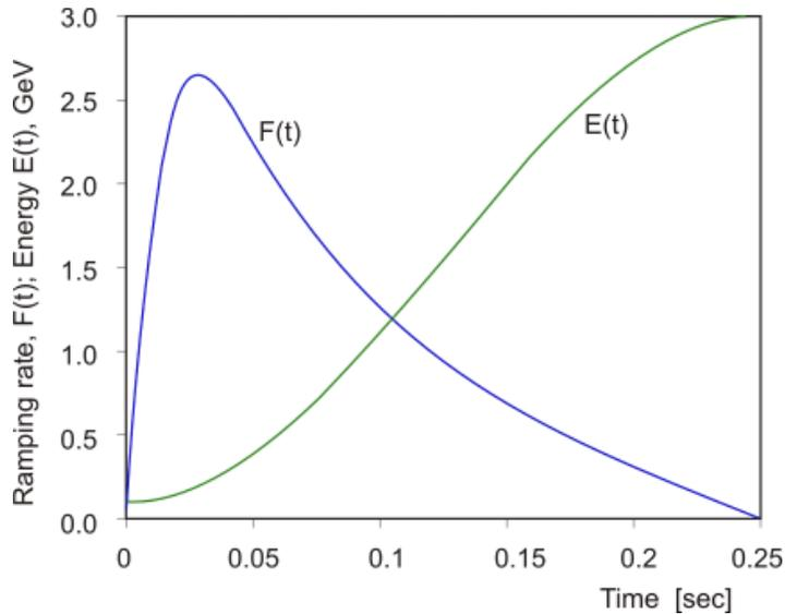
**Fig. 4.2.6 Dipole field ramping rate and beam energy variation during the ramp.**
