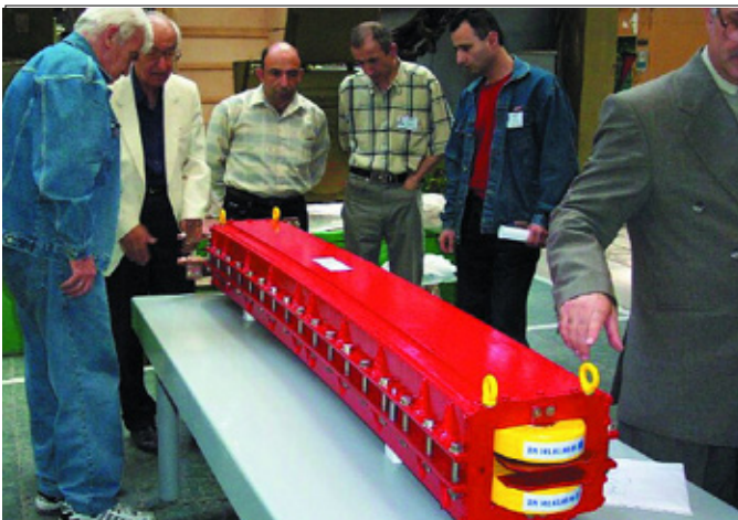
The first prototype dipole magnet for the CANDLE booster ring.
