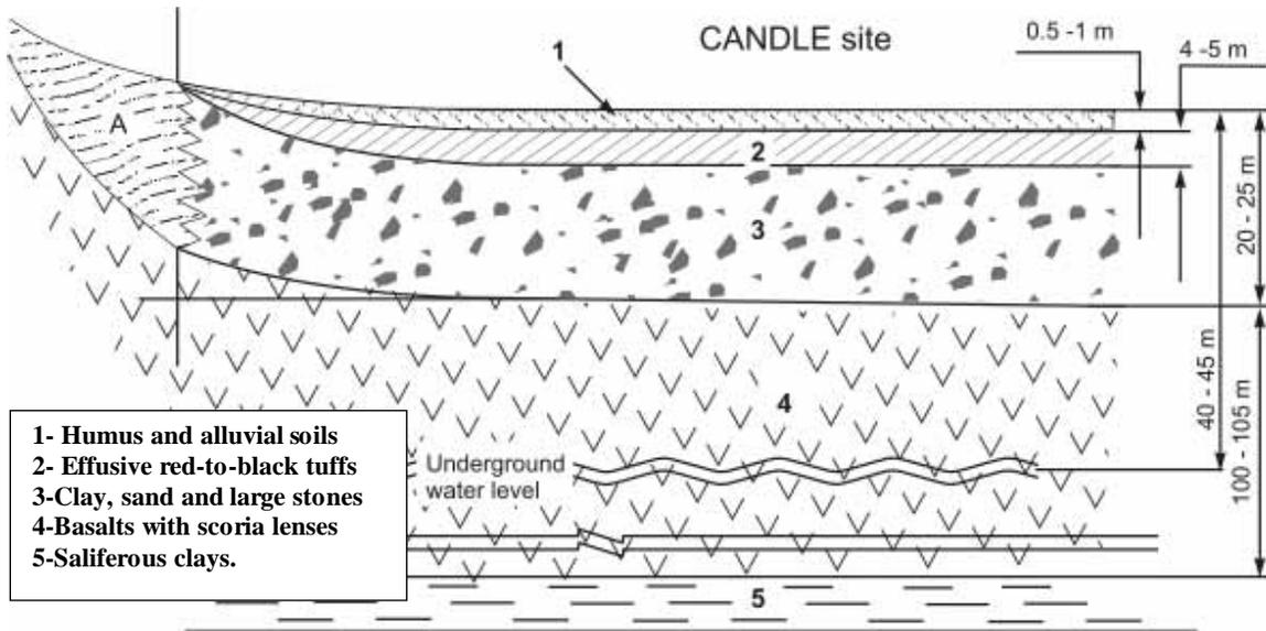
**Fig. 8.1.1 Geological structure of the ground at the CANDLE site.**
