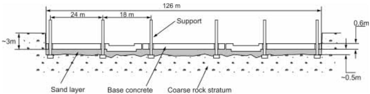
**Fig. 8.2.4 The building base construction approach.**
