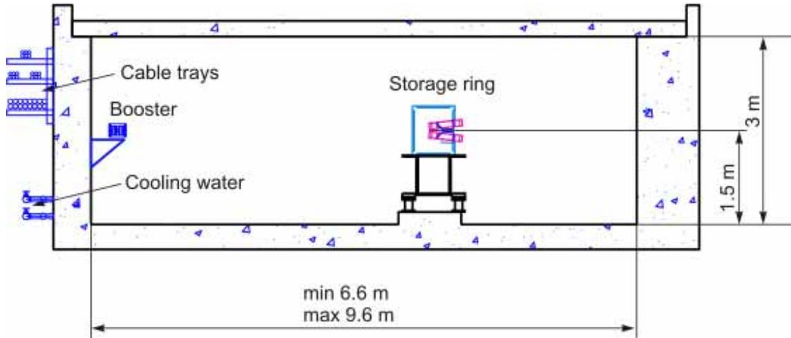
**Fig. 8.2.2 Accelerator tunnel and utilities.**
