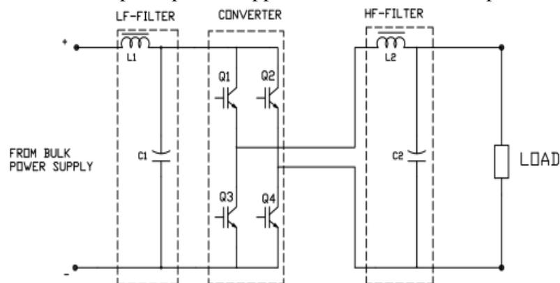
**Fig.3.9.6 The correction magnet power supply principal diagram.**
