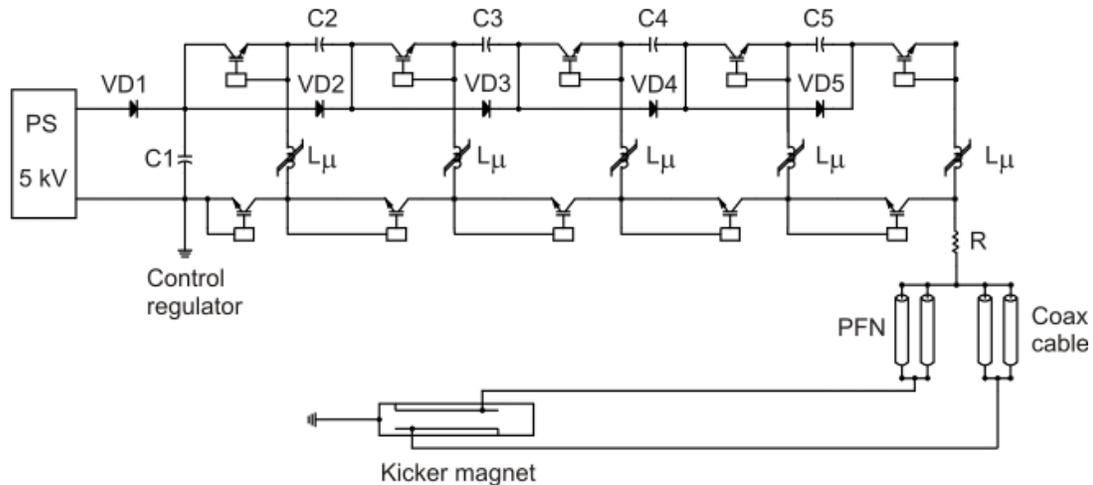
**Fig. 3.9.9 Kicker magnet power supply scheme.**
