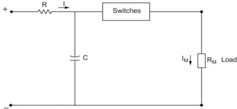
**Fig. 3.9.7 The pulse generator general scheme.**
