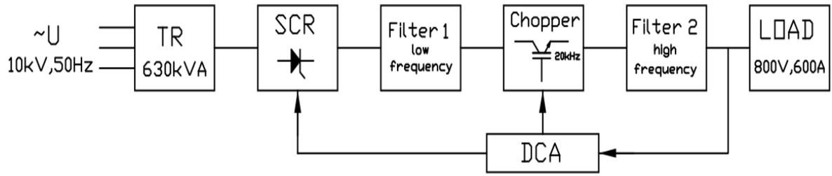
**Fig. 3.9.1 The power supply scheme for the 32 dipoles.**
