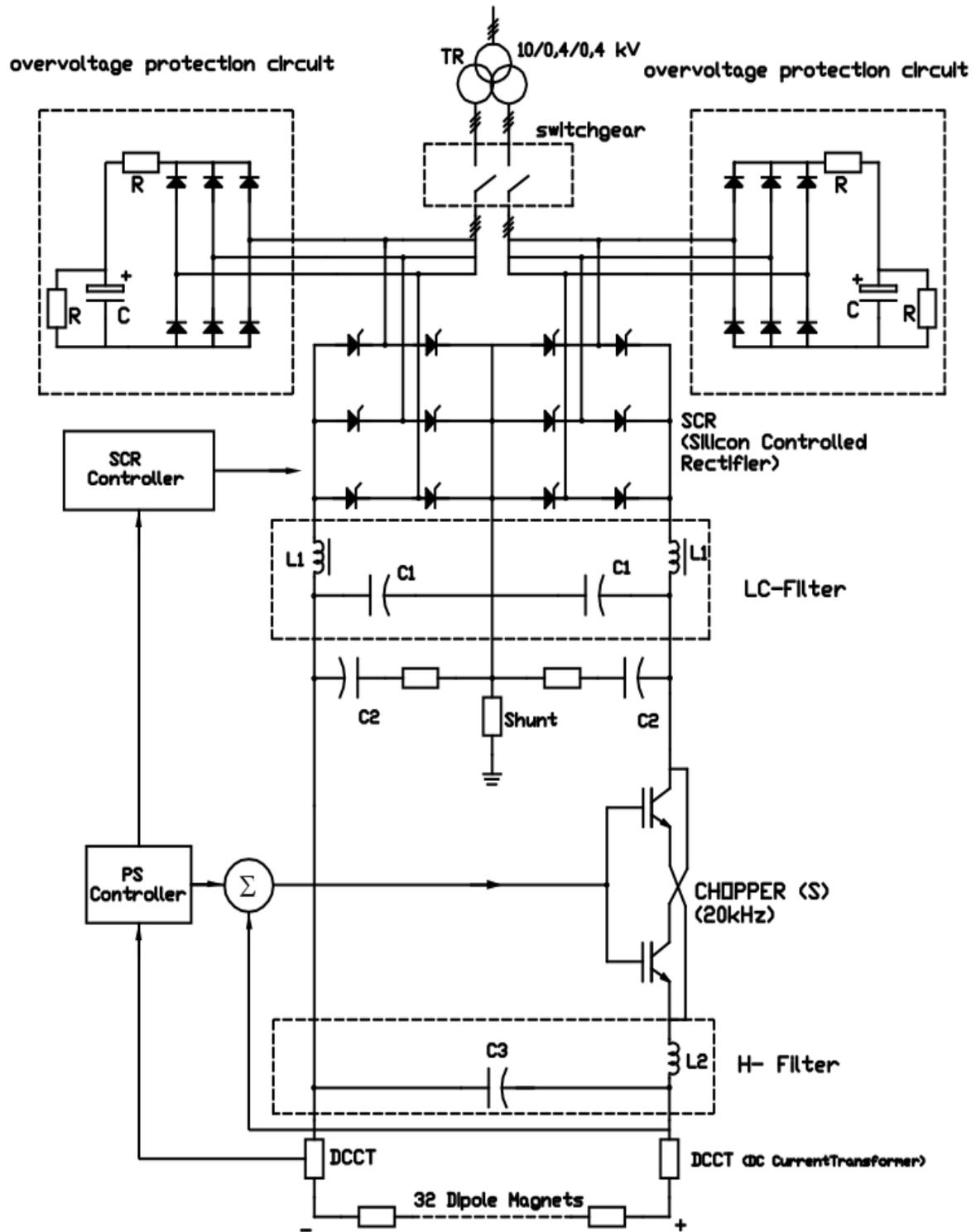
Fig. 3.9.3 Dipole magnets power supply circuit diagram.
