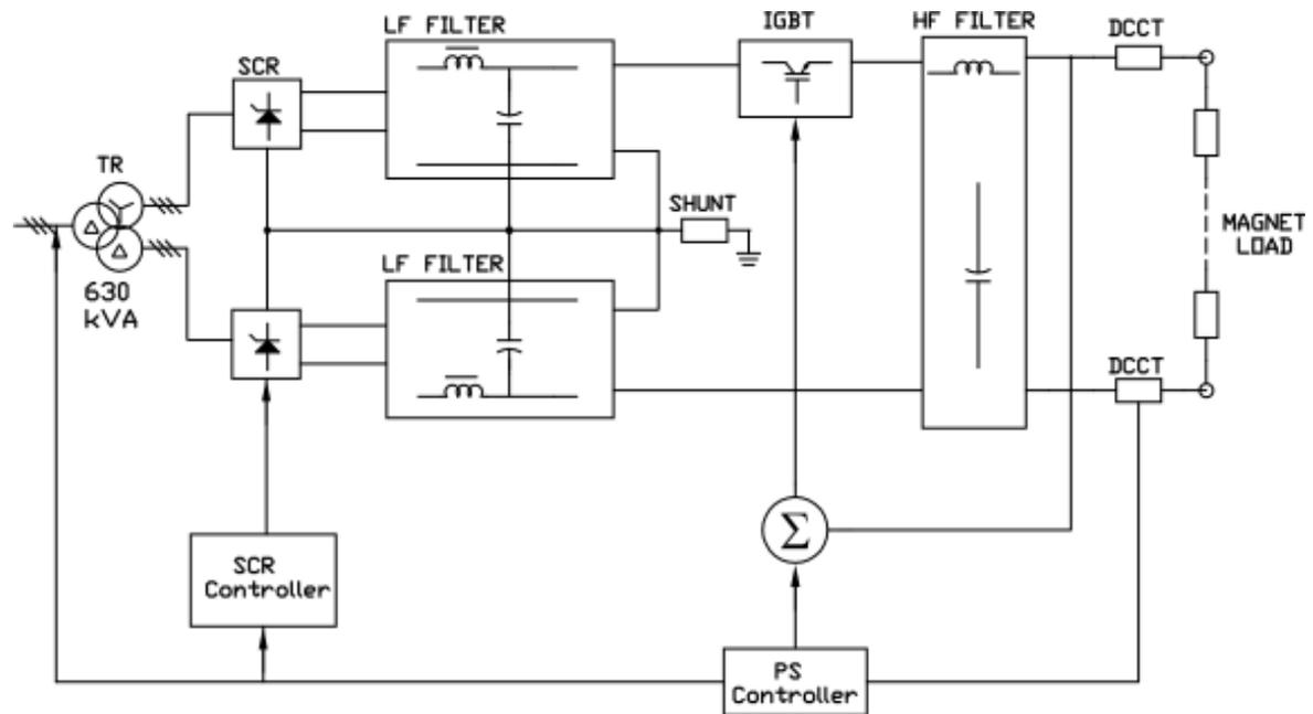
**Fig.3.9.2 The block diagram of dipoles power supply.**
