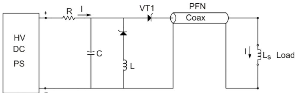
**Fig. 3.9.8 The septum magnet power supply principal scheme.**
