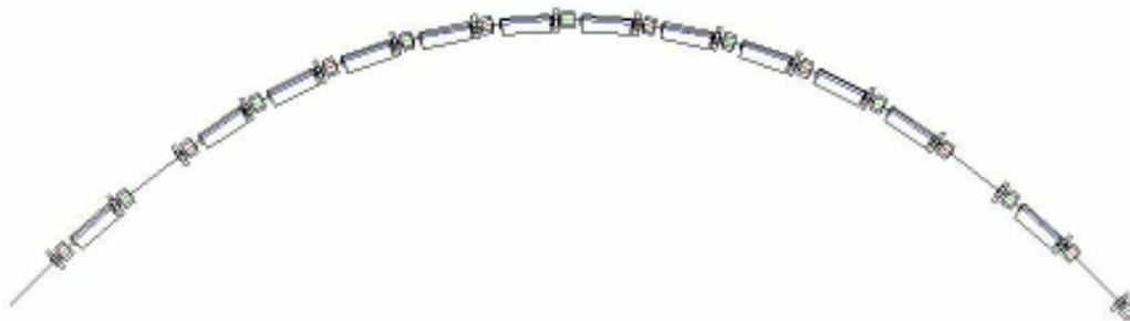
Fig.4.1.2 Schematic layout of the one quadrant of booster lattice.
