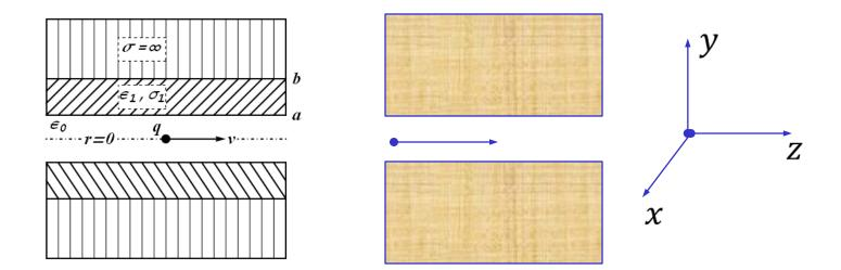
$$E_z(q,k) = \frac{Z_0}{16\pi^2} \frac{k \left(K^2 - q^2\right) Sh(2dK)}{\left(KCh(Kd)Ch(qa) - qSh(Kd)Sh(qa)\right) \left(q(q^2 + k^2 - K^2)Ch(Kd)Ch(qa) + kK^2Sh(Kd)Sh(ka)\right)}$$
