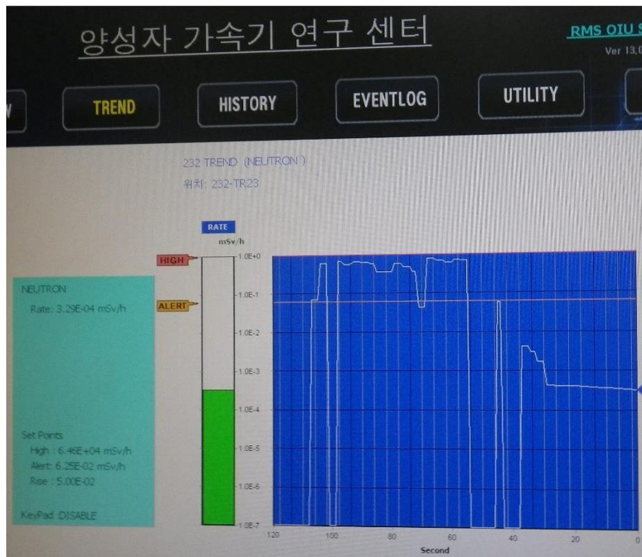
The proton beam indirectly was measured by neutron detector (type ?) mounted outside from beam path. Before VWM the proton beam was marked by this detector only. **Not all events from this detector are attended to real beam measured by VWM!!!**
