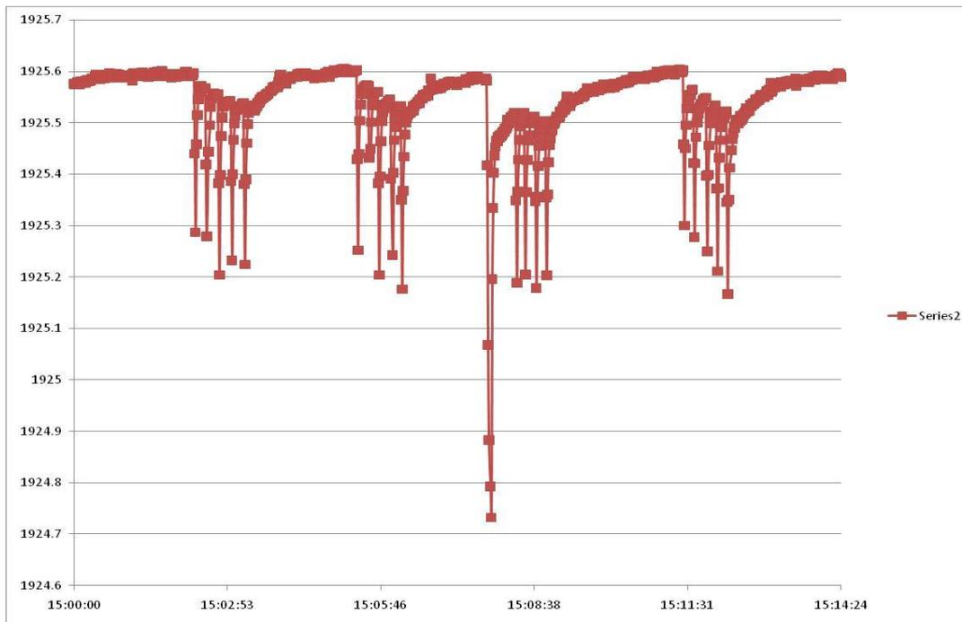
Different series of pulses. The first and fourth are more regular in time and amplitude of the peaks, in the second the second train is obviously weak, in the third we saw non regular time structure of trains.
