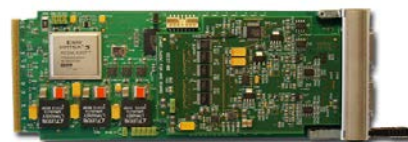
TEWS TAMC100 IP Carrier with DESY IP timer board
