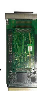
TEWS TAMC100 IP Carrier with DESY IP timer board
