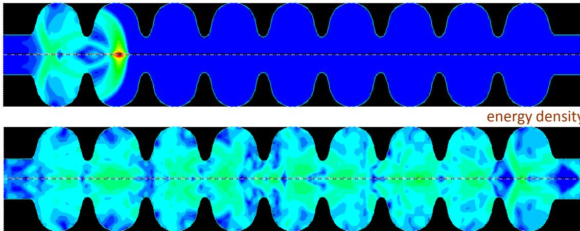
eigenmodes are excited and ring forever (if there is no damping)
