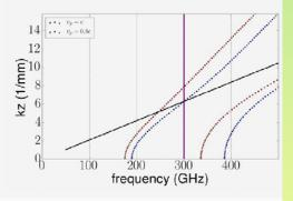
Dispersion curve for quartz DLWs with different thicknesses for same inner radius of 0.5 mm. The solution corresponding v p = c is illustrated in blue dots with corresponding dimension (a, b, r) = (0.5 mm, 0.590 mm, 4.41), the red dots correspond t a solution for v p = 0.8c with corresponding structure (a, b, r) = (0.5 mm, 0.612 mm, 4.41).
