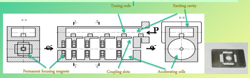
Prototype structure with 2450 MHz
