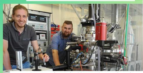
Development of reproducible growth procedures for photocathodes with high quantum efficiency, smooth surface and long operational lifetime.
