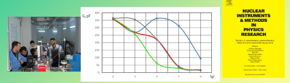
**Before-blue line**; after the first irradiation-red; after the second irradiation-green; after the third irradiation-purple. AREAL Ultrafast Beam Application for Modeling the Microorganisms Survival in Space Garnik Khachatryan (YerPhI)
