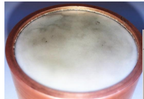
Alumina to Cu brazing Mo wire fixation
