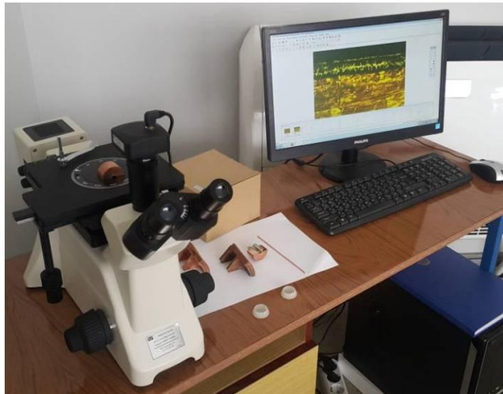
Figure 2.4.1.-5: Metallurgical microscope.
