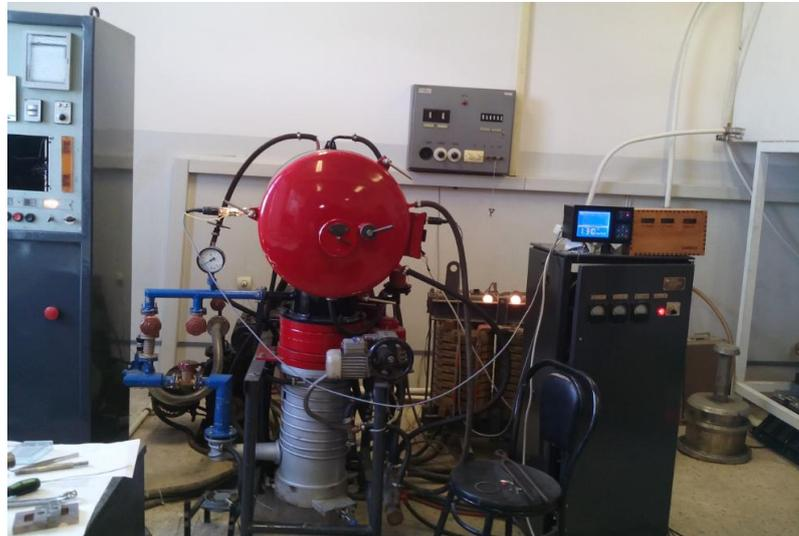
Figure. 2.4.1.-1: The vacuum furnace.
