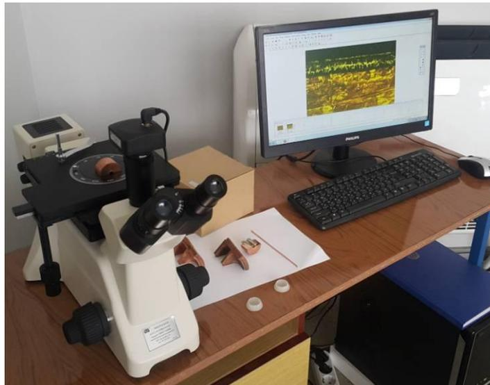
Figure 2.4.1.-5: Metallurgical microscope.
