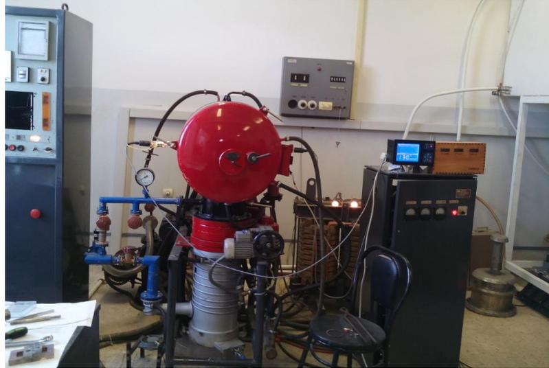
Figure. 2.4.1.-1: The vacuum furnace.
