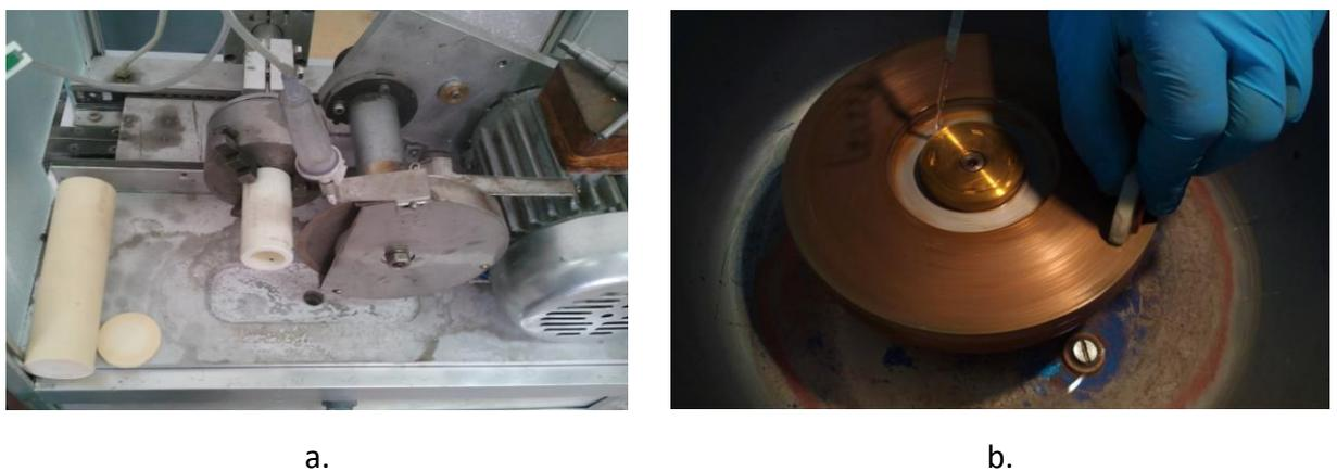
Figure.2.4.1.-4: a. Diamond machining machine, b. diamond polishing disc.
