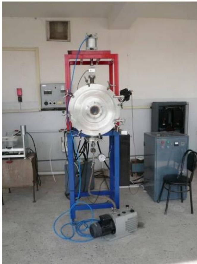
Figure 2.4.4: Diffusion welding machine.
