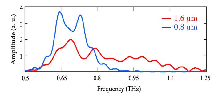
Spectrum of the multi-cycle THz pulse in APPLN with  $\delta$  = 0.8 µm lies in range of 0.6-0.8 THz that is beneficial for THz waveguide based particle acceleration.
