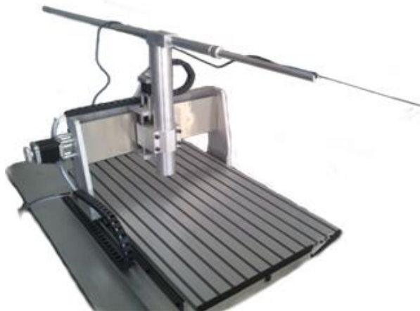
Figure 5.1: Magnetic Measurement Bench; the maximum movement along the directions is x = 40cm , y = 90cm , z = 14cm , where z is directed along the robotic arm. The minimum step is 10^{-4}cm .
