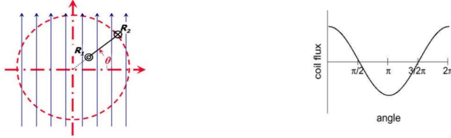
Fig. 3.2: 2D representation of the flux seen by a simple coil rotating in a dipole field
