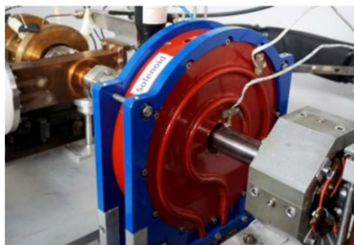
Figure 4.13: The quadrupole magnet is mounted downstream to the solenoid magnet for
