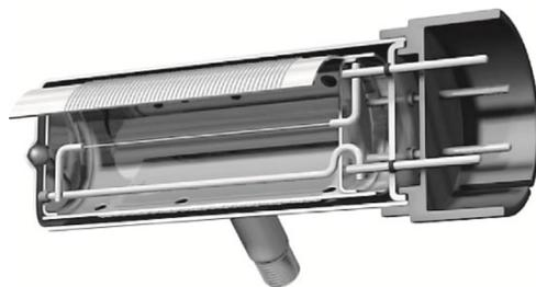
Figure 6.17 Section of a measuring tube in a thermal conductivity vacuum gauge (constant wire temperature) with gold-plated tungsten heating wire and a measuring range from 0.1 Pa to 100 kPa. The surrounding cylindrical housing (see heating wires) is temperature controlled to approximately 40 °C for increased measurement accuracy. At higher pressures, heat transport due to convection is used as a measuring signal.
