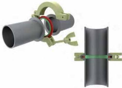
Figure 7.10 ISO-KF connection with centering ring and clamping ring
