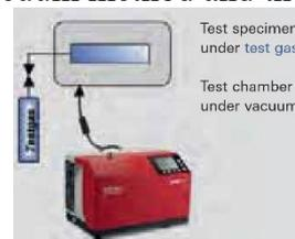
Figure 8.14 Integral leak detection of enclosed objects with the sniffer method
