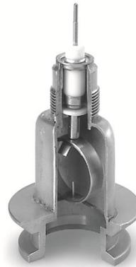
Figure 6.38 Penning gauge. (Courtesy of INFICON Inc.)
