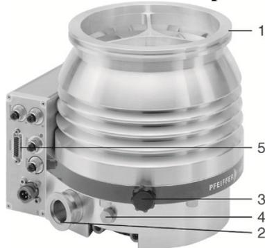
Figure 5.12 Single-flow turbomolecular pump HiPace 700 by Pfeiffer company with attached drive electronics for 48 V DC. 1: high-vacuum flange; 2: fore-vacuum flange; 3: venting valve; 4: purge-gas port; 5: electronic drive unit with remote control socket.
