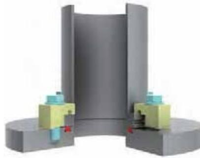
Figure 7.14 ISO-K flange mounted on base plate with O-ring nut and claw clamps for base plate with sealing groove
