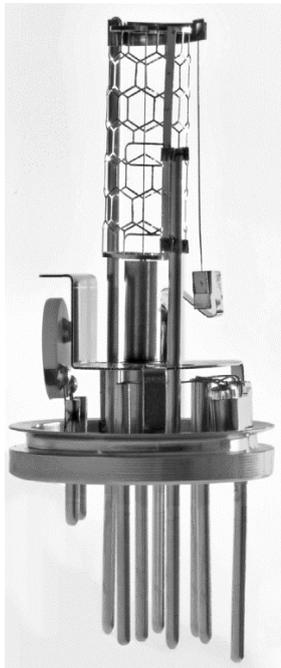
Figure 6.44 Combined vacuum gauge BCG 450 by INFICON with a range from  $5 \times 10^{-8}$  Pa to 150 kPa.
