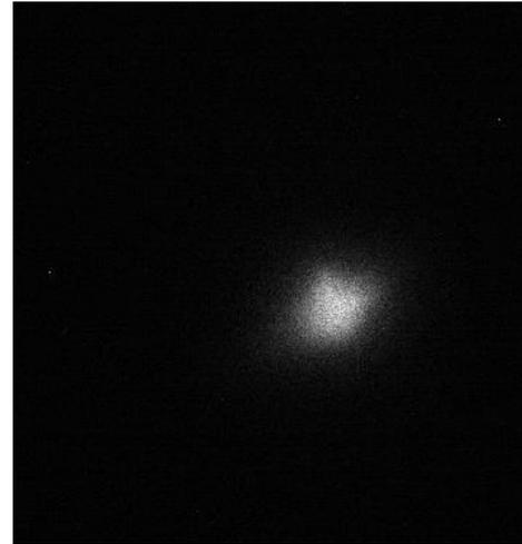
REGAE electron beam on YAG-screen
