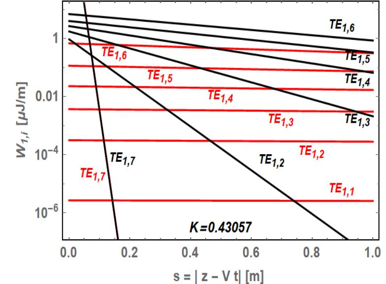
The dependence of the accumulated energy density on the distance to the particle, TE modes,  $n = 1$ ; radiation forward (black lines) and backward (red lines).
