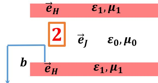
Matching the tangential components of full field on the inner wall at  $r = b$
