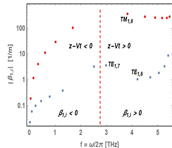
Damping factors of TE (blue) and TM (red) modes at resonant frequencies for  $n = 1$ .
