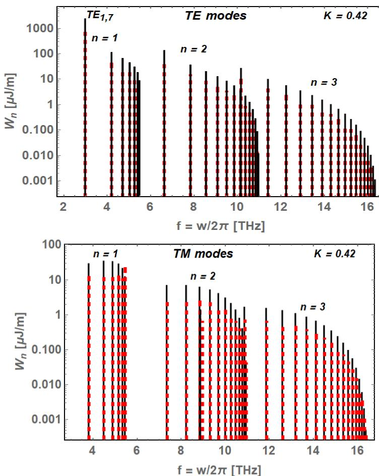
Spectral distribution (space-time domain, forward direction,  $z - Vt \rightarrow 0$ ) of first three multipoles ( $n = 1,2,3$ ) stored radiation energy for TE (top) and TM (bottom) modes in a copper (red, dashed) and ideal (black, solid) waveguides.
