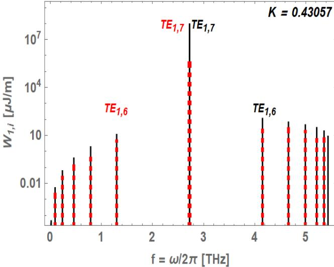
Spectral distribution (space-time domain) of dipole mode ( $n = 1$ ) stored radiation energy for TE modes in a copper (red, dashed) and ideal (black, solid) waveguides.
