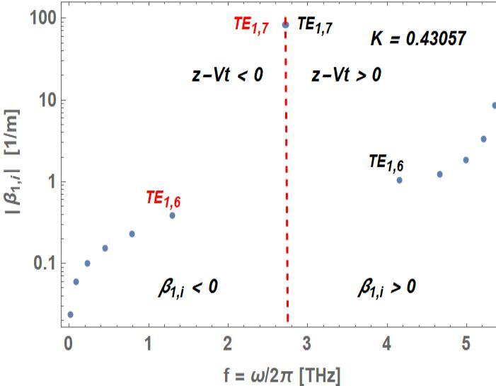
Damping factors of TE modes at resonant frequencies for  $n = 1$ .
