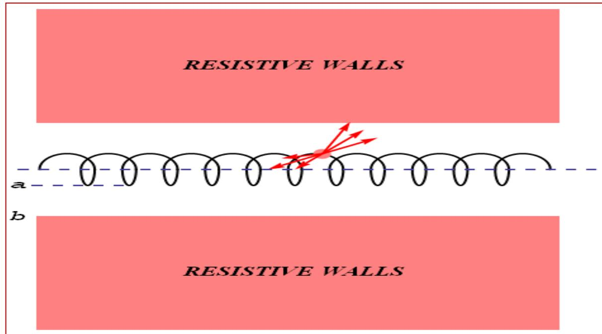
*The radiation field of a particle moving on a helical trajectory in a cylindrical waveguide with resistive walls is calculated.*
