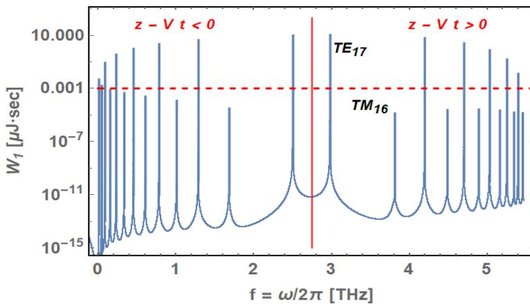
Spectral distribution of dipole mode ( $n = 1$ ) radiation in a copper waveguide; forward (right) and back (left) radiation.
