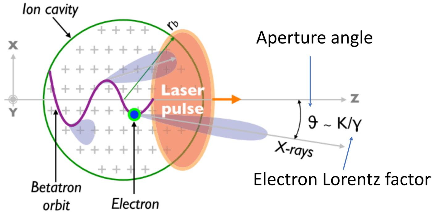
Undulator parameter  $K = \gamma k_{\beta} r_{\beta}$  ← Oscillation amplitude
