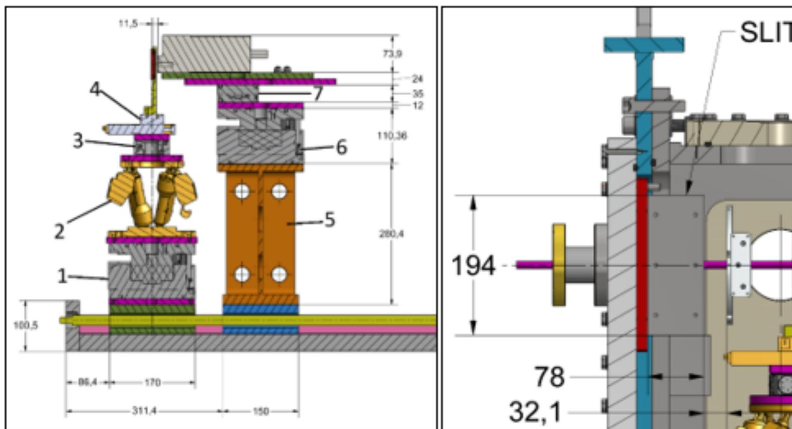
Figure 3 - Diagram showing the most important components other than the x-ray Camera and the sample holder system (left), and the slit system (right), with distances expressed in mm. The numbered components are explained in the text.
