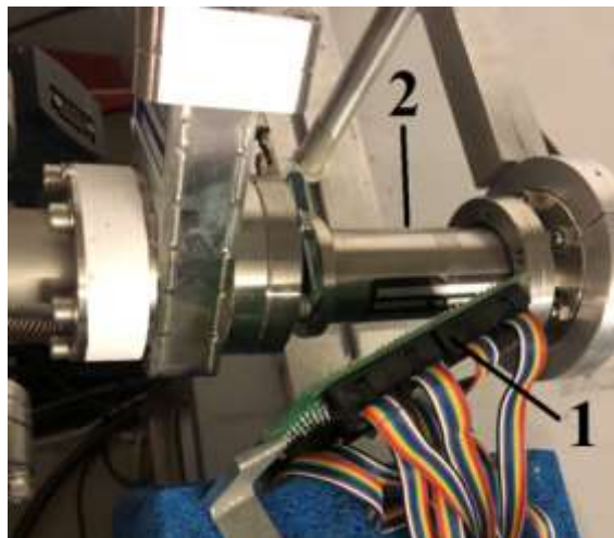
1 - Faradau cup, 2 - PIN-photodiode array
