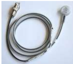
Dose-1 Dose Meter with NACP-02 ionization chamber
