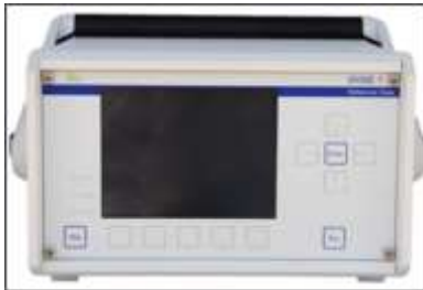
Dose-1 Dose Meter with NACP-02 ionization chamber
