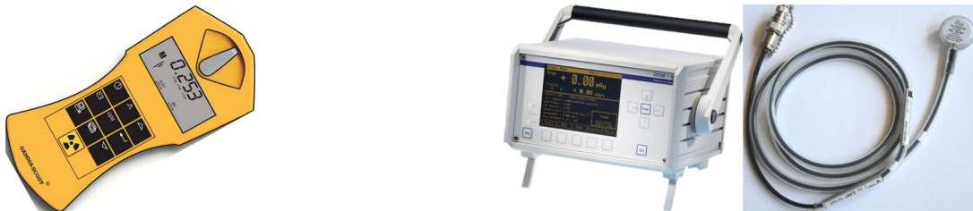
(a) GAMMA-SCOUT, a Geiger-Mueller radiation detector. (b) The high-precision electrometer DOSE-1 (left) and the ionization chamber NACP-02 (right).
