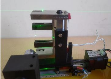
Left: general view of test bench of VWM eqipped with stepper motor feed. As a beam the semiconductor laser is used. The monitor is covered with a box to protect it from convective air streams
