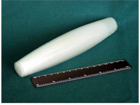
4 th - monolithic lens made of Poly capillaries
