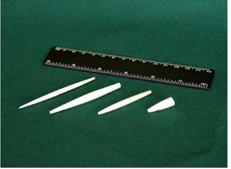
4 th - monolithic lens made of Poly capillaries
