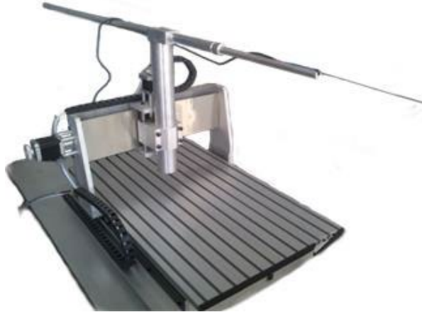
Figure 6.1: Magnetic Measurement Bench; the maximum movement along the directions is x = 40\text{cm} , y = 90\text{cm} , z = 14\text{cm} , where z is directed along the robotic arm. The minimum step is 10^{-4}\text{cm} .
